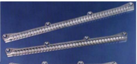
Die-cast ACuZinc replaced P/M for these gear racks and provides greater wear resistance and strength. The racks are produced in lengths of 255 mm, 300 mm and 340 mm.
