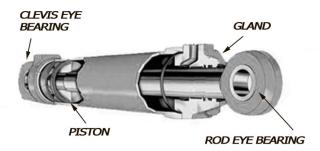
Many hydraulic cylinder components are traditionally made of bronze. These include cylinder eye bearings, gland or rod bearings and various internal components such as piston heads, cushions and guides.
