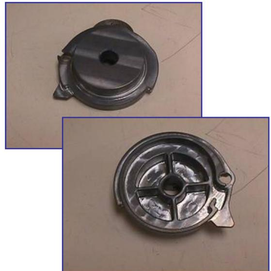
Figure 2 –Emergency Brake Drum machined from Zamak 3 Con-Cast Bar Stock
