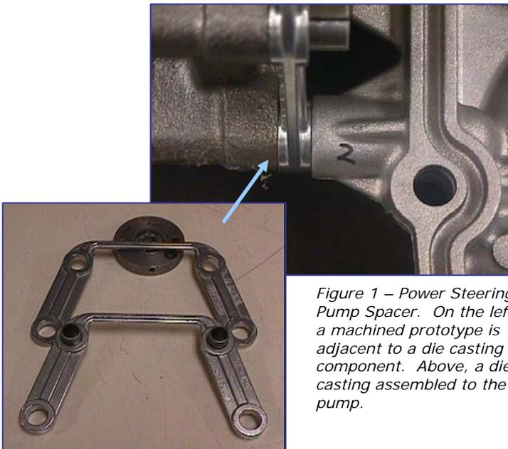
Figure 1 – Power Steering Pump Spacer. On the left, a machined prototype is adjacent to a die casting component. Above, a die casting assembled to the pump.
