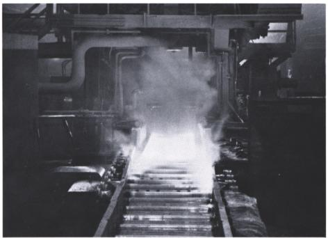
ZA-12 zinc runout table bushings replaced bronze in a steel hot mill environment. Table rollers are seated in ZA-12 bearings and support fast moving hot steel from breakdown mill similar to above. Zinc bearings provided service life double that of bronze.
