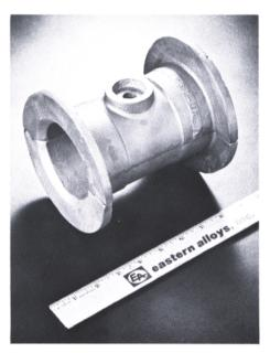
Typical split flanged ZA-12 steel mill table bearings now used by Crucible Inc., Midland, Pa. Zinc bearings provided longer service life and superior emergency running (no lubrication) characteristics at lower cost than bronze.
