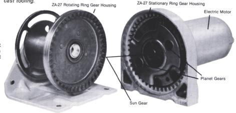
Efficient Superwinch design shows sun gear, driven by electric motor, and plant gears which revolve against 5-inch diameter die-cast ring gear housings (stationary and rotating). ZA-27 and aluminum parts are made in the same die-cast tools. ZA-27 components are used only in high-load winch modes where the superior strength and natural lubricity of ZA-27 is required.
