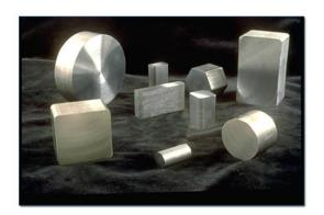
For the majority of applications, using the same con-cast alloy to prototype for a die casting is sufficient; however, some properties such as creep resistance or ductility may not be as similar. In these cases, please call us for other solutions to your prototyping needs.
