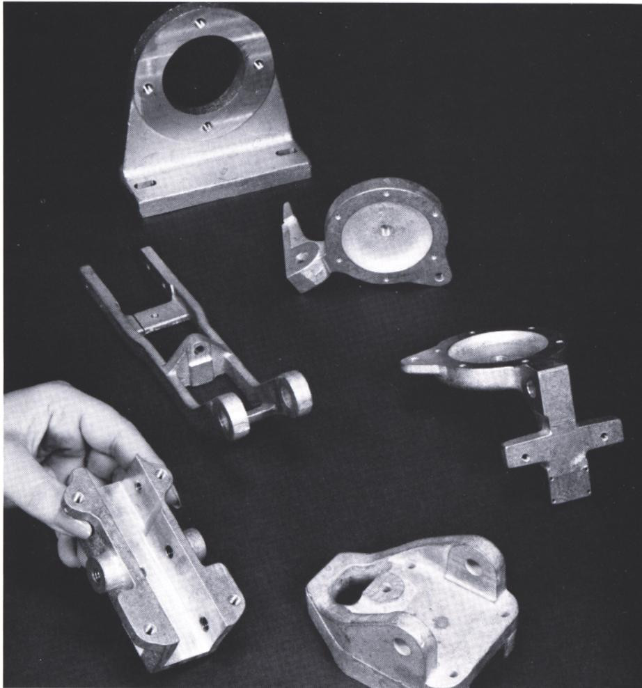
ZA-12 castings provide excellent wear resistance, high strength and pressure tightness.
